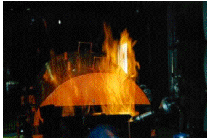
(d) Lance unit during flame hardening of the pipe.
